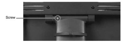
**5** Remove the four small screws from the back of the LCD panel. Do not discard the four screws.
